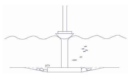
Figure 1. Schematic drawing of a gravity-based foundation made of concrete (scales and dimensions are not proportional).
